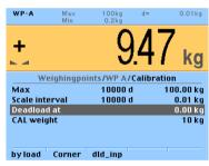
No need to enter load cell parameter load cell position
